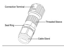
a) Lead the AC cable though cable gland, seal ring and threaded sleeve, and fully insert the conductors to corresponding terminals on connection terminal
