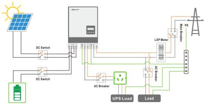
Please prepare the breakers before connetion, breakers selection recommendation for both DC and AC
