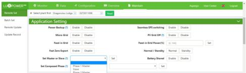
Step4. Enable share battery for the system if the system share one battery bank, otherwise disable the shared battery function
