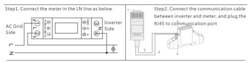
Step3. Check the connection. When the meter displays -xxxxW as below figure shows, the hybrid inverter is feeding power to the grid.and when it displays xxxxW, it means the house load is using energy from grid.
