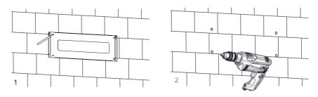
**Step2.** Install the expansion tubes into the holes and tight them, then use the expansion screws (packaged together with the expansion tubes) to install and fix the wall-mounting bracket on the wall.
