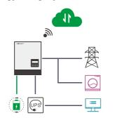
C. On-grid solar system without battery (hybrid ready)
