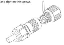
b) Refer to below figure and confirm the AC cables are correctly connected. The difference between the AC connector and UPS connector is that AC connector housing engage perfectly until a 'click' is heard or felt. has a "Grid" mark on it and UPS does not
